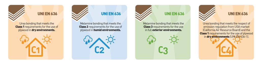
Plywood is used in many application areas, such as structural bracing, concrete formwork, cladding, flooring, webbed beams, boats, aircraft, door skins, furniture, wall panels and architectural joinery in exterior and interior environments. The ratio between thickness and number of layers (veneers) affect the glue quantity per m<sup>3</sup> necessary for bonding.
